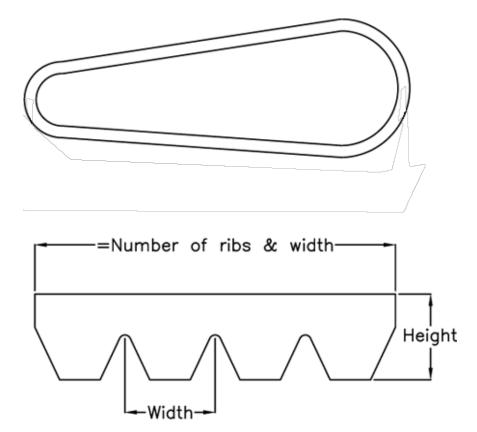
$\begin{array}{ll} \text{Datum Llength} = 1910 \\ \text{Height} &= 3.5 \\ \text{Number of ribs} = 9 \\ \text{Pitch} &= 2.34 \end{array}$
